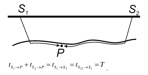
which is the *reciprocal travel time* corresponding to wave propagation from one source point to another. Note that this method works even for varying interface depth between the shot points.
