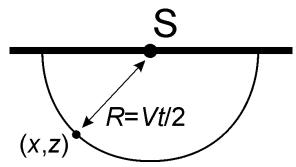
Conversely, the reflectivity at depth point (x,z) can be determined by adding the amplitudes from all the sources (=receivers) **S**, each taken at time t=2R/V, where:
