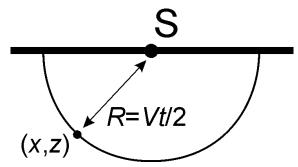
Conversely, the reflectivity at depth point (x,z) will be recorded from any source (=receiver) **S** at time t = 2R/V, where the distance *R* varies with  $x_s$ :
