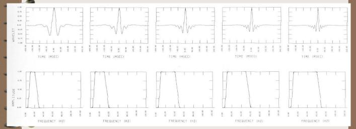
• Equal-amplitude (co)sinusoids from 0 to  $f_N$  add up to form a spike:
