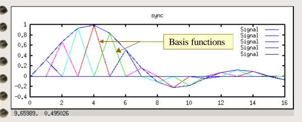
• Fourier transform represents the signal as a sum of sin(...), cos(...), or complex exp(...) basis functions with different *frequencies*:
