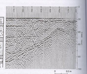
Although converted into depth units, this is still a *time section*! So, geometry of bedrock walls is not accurate...
