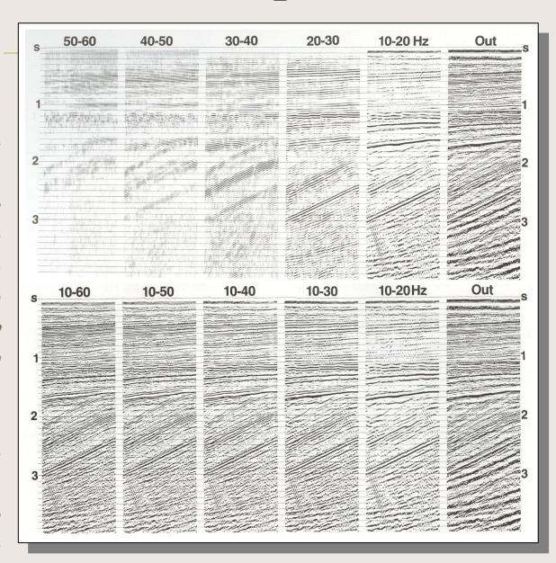
• Trial band-pass filter panels are designed in order to determine the best frequency range for data display and analysis. For a final display, *time-variant* filters are used.
