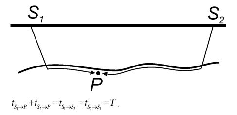
This sum T equals the <u>reciprocal travel time</u>, which is the time of head-wave propagation from one source point at the surface to another one. Regardless of the shape of the refractor or surface topography, these times from source  $S_1$  to  $S_2$  and backward are equal. The reciprocal time can be easily read from the travel-time curves you drew in Method 1 above.
