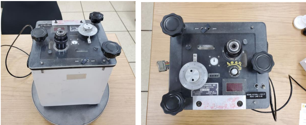
Figure 1. Lacoste G267 relative gravimeter used in this lab
