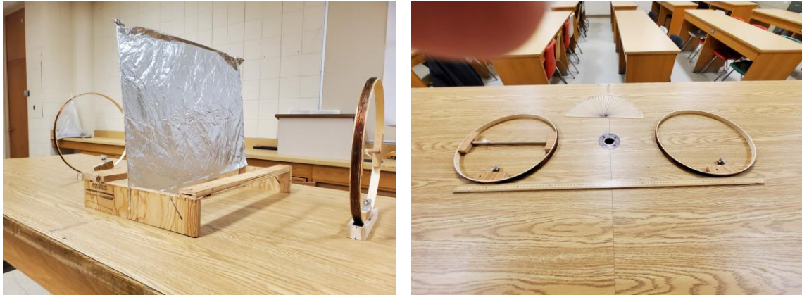
Figure 4. Transmitter and receiver coils used in the measurements, in vertical (left) and horizontal (right) arrangements.
