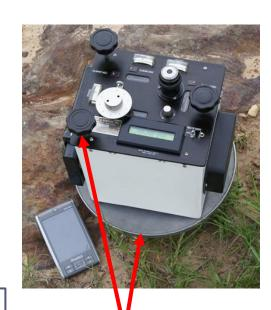
Leveling plate and knobs
