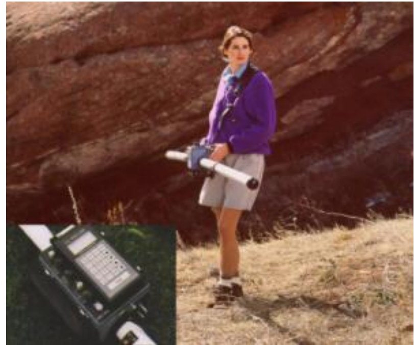
EM31 : Sounding depth ~6 m Intercoil spacing 3.6 m, Frequency 9.8 kHz
