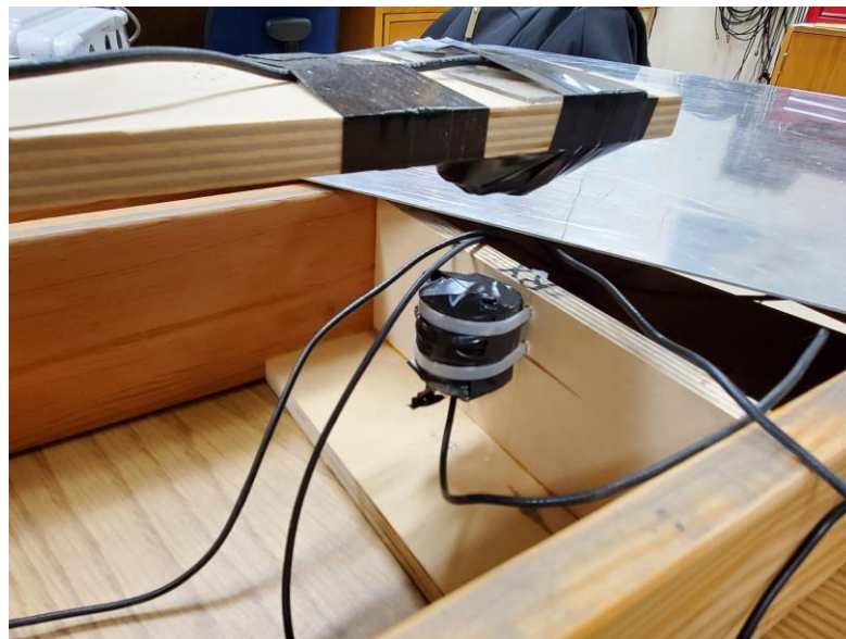
Figure 1. Skin depth experiment: a) operational assembly; b) zoom-in with the metal sheet removed. The Tx and Rx coils wrapped in black electric tape. The Tx coil is placed above the sheet, and Rx is below it.
