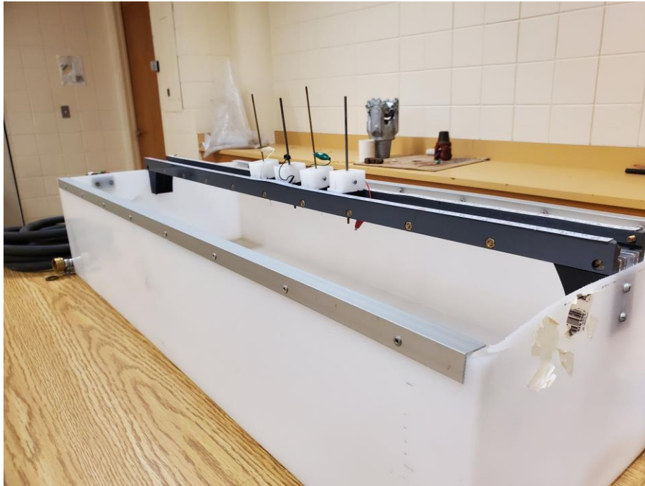
Figure 1. Electrical modeling tank in Geology 265. Note the four electrodes on top in an A-M-N-B configuration for Wenner sounding
