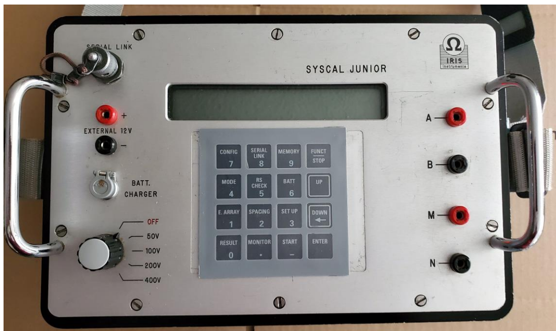
Figure 2. SYSCAL Junior resistivity/IP/SP meter used in field schools and labs.
