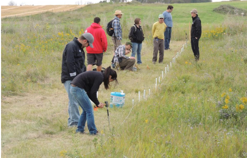
Figure 1. Small IP survey during Geophysics field school 2012. White ceramic tubes are the nonpolarizable electrodes
