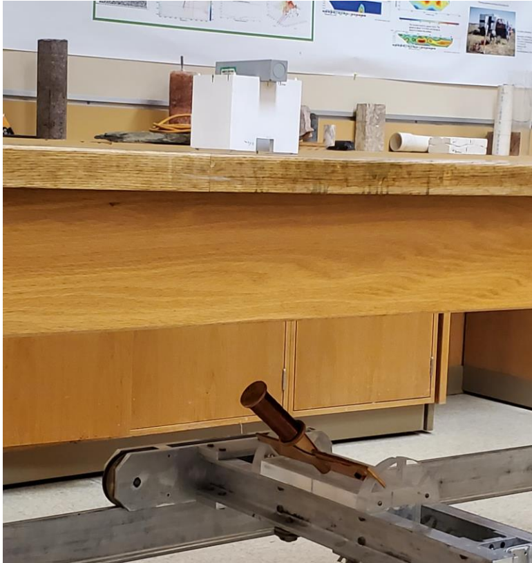
Figure 2. Dipole magnetic source (coil of copper wire) in tilted at 30^\circ position and sliding along rails on the floor.
