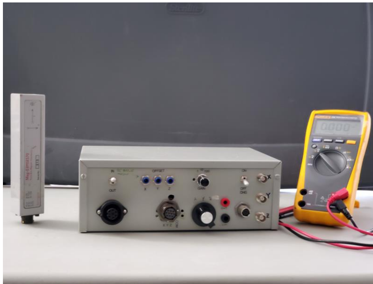
Figure 1. Fluxgate magnetometer (left), its receiver (middle) and millivoltmeter for data recording.
