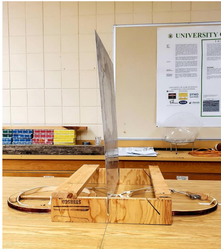
Figure 2. Transmitter and receiver coils, and the target (aluminum sheet).
