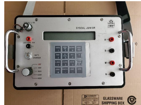
SYSCAL resistivity meter used in our field schools and labs
