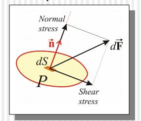
At point P, force  $d\mathbf{F}$  acts on any infinitesimal area dS.  $d\mathbf{F}$  is a projection of stress tensor,  $\sigma$ , onto  $\mathbf{n}$ :
