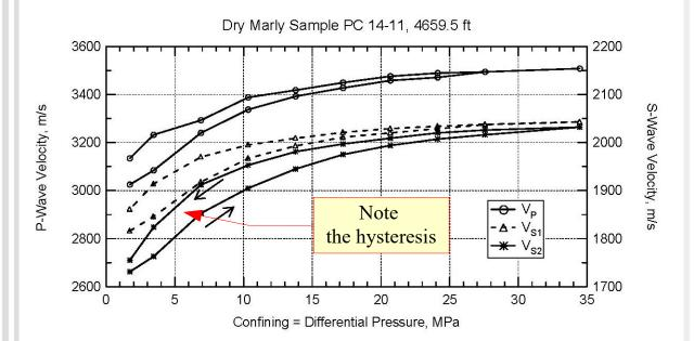
Dry carbonate sample from Weyburn reservoir
