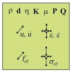
The state of effective medium is described by average displacement **u** and displacement rate  $\dot{\mathbf{u}}$ , which produce drag friction force  $\mathbf{f}_{\text{eff}}$  and stress  $\boldsymbol{\sigma}_{\text{eff}}$
